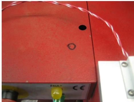
14. Take **ONE** of the wires soldered to the back of the E-Switch and cut the wire half-way between the E-Switch and where the wire runs back into the mill.
