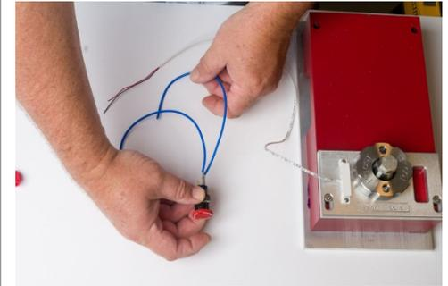
12. Locate and drill a 1/4" hole in the top of the control box 1" from the side where the control box meets the belt cover and 1.5" from the front edge of the control box. Deburr the hole and install the supplied black rubber grommet in this hole. Run the wire leads from the Safety Switch through this grommet into the Control Box.
