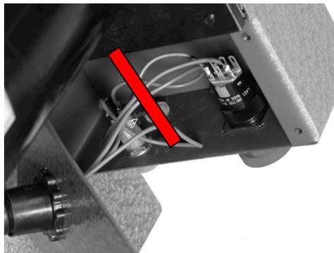
15. Using the supplied wire connectors, splice the Safety Switch between the ends of the E-Switch wire cut in the previous step.
